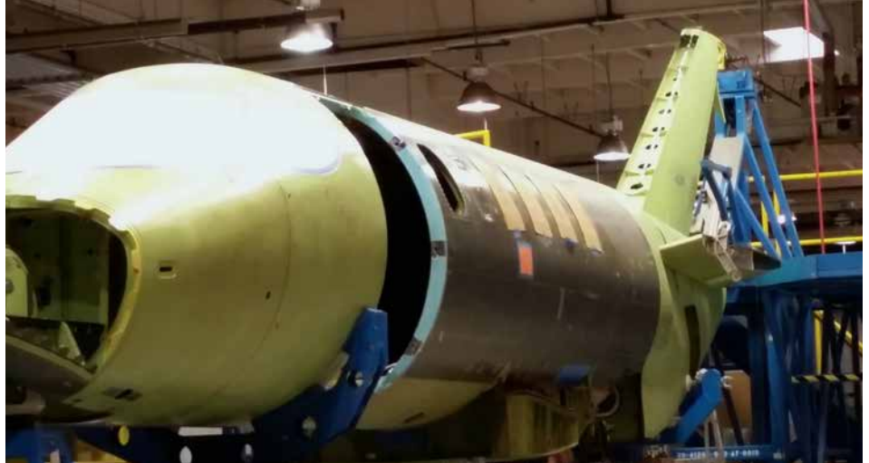
Serial number 012 with vertical tail mated in Cedar City production facility.
